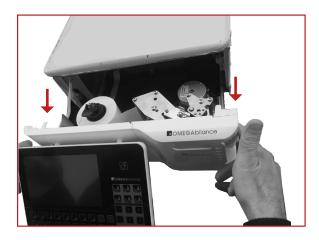
**3.**Open the print head assembly by turning the lever
