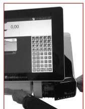
**3.**Lift the lever and pull out the paper
