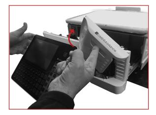
**4.**Lift the lever and pull out the paper
